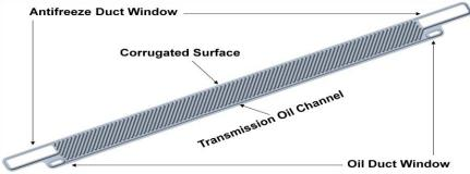
\*\* Saved space can be used for additional heat transfer or other components (intercooler, engine oil cooler, a/c condenser, etc). TPT manufacturing process can accommodate any shape (circle, rectangle, oval, etc).
